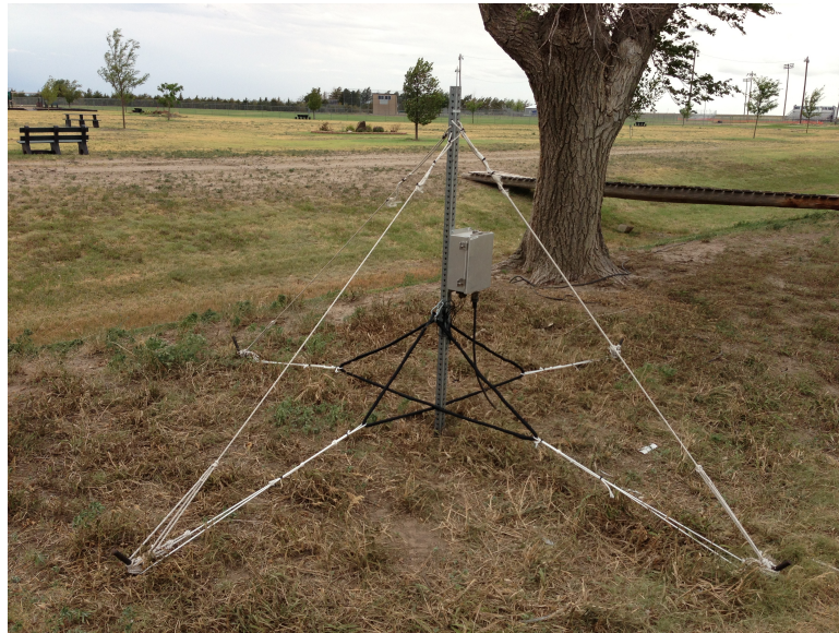
Figure 2.7: A photograph of a VLF/LF receiver loop antenna used in the Oklahoma array.
