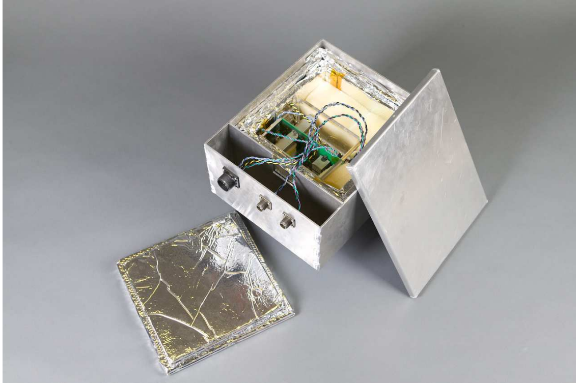
Figure 7.2: Photo of preamp box including preamp board and insulation. Each box includes two analog channels.
