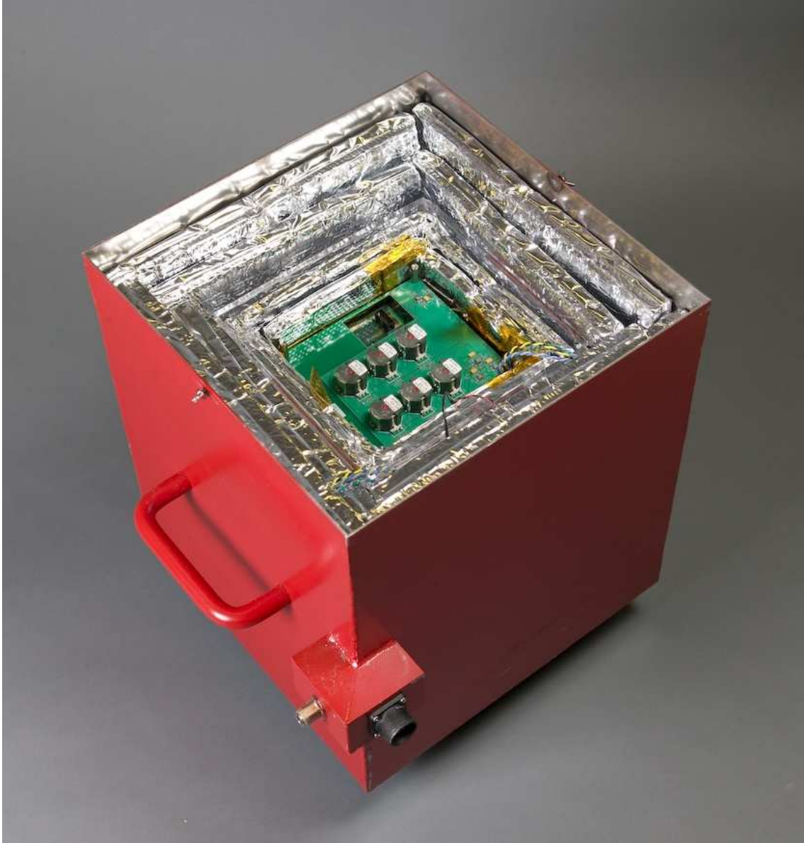
Figure 7.6: Photo of digital box, which includes the battery back, digital card with storage, and the filter card. Only the filter card is visible.
