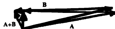
Fig. 10. When two strong signals propagating in different modes (represented by vectors A and B) combine in a destructive manner (i.e., a small difference between large values), small changes in each mode (from the original grey vector to the new black vector) can result in large phase changes and large relative amplitude changes in the sum.
