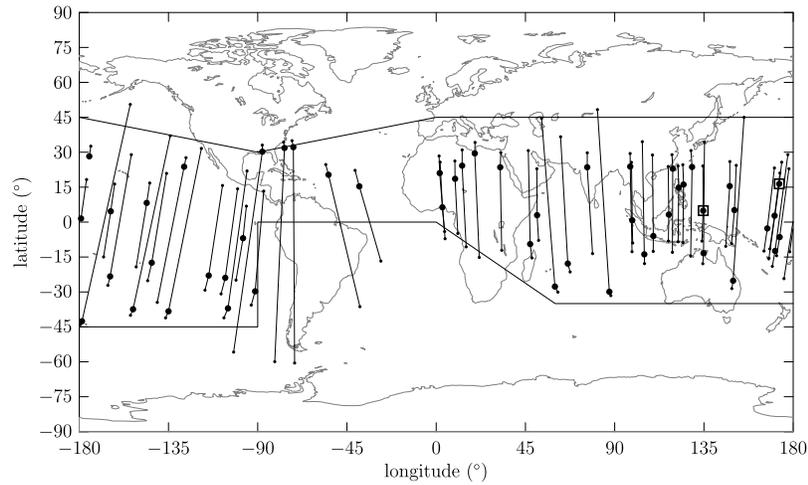
**FIGURE 3.** Geographic location of the satellite when events were observed. Large dots represent the satellite location, with the satellite's north and south geomagnetic footprint indicated by small dots connected by lines to the associated satellite location. The lines running across the map isolate the region below the radiation belts where the search was executed.
