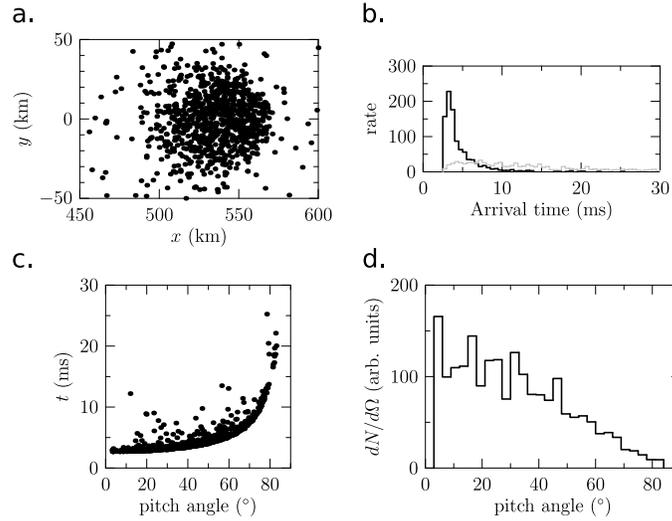
**FIGURE 1.** Results of simulations of properties of electrons emitted along with photons in a TGF. Properties shown when electrons first reach satellite altitude. a. distribution in plane at satellite altitude. b. arrival time distribution at satellite altitude (black), arrival time distribution spread out by a factor of 10 (grey). c. arrival time as a function of pitch angle. d. pitch angle distribution.
