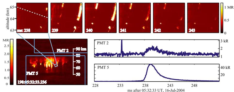
**Figure 1.** Sprite event of 05:32:33 UT, July 16, 2004. The top six panels show consecutive frames of the high-speed imager; the bottom left shows the wide field-of-view sprite image and the relative location of the narrow field-of-view; the bottom right shows two channels of photometer data. Note that Rayleigh intensities in the photometer channels are averaged over the photometer field-of-view, which is much larger than the sprite.
